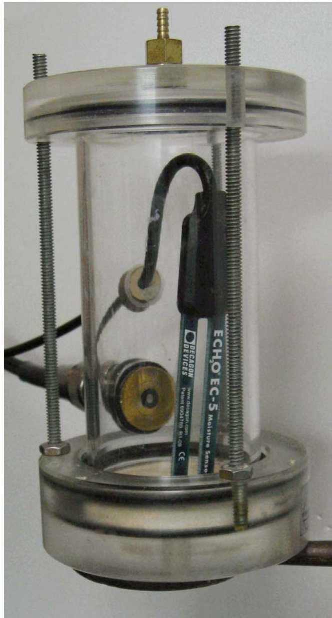
Figure 13. Modified Tempe cell designed to provide soil permittivity measurements to coincide with draining water retention measurements. Pressure was applied in steps to the cell to force water out the bottom through a ceramic plate. A water content sensor was also included in the cell for independent measurements of volumetric soil water content.
